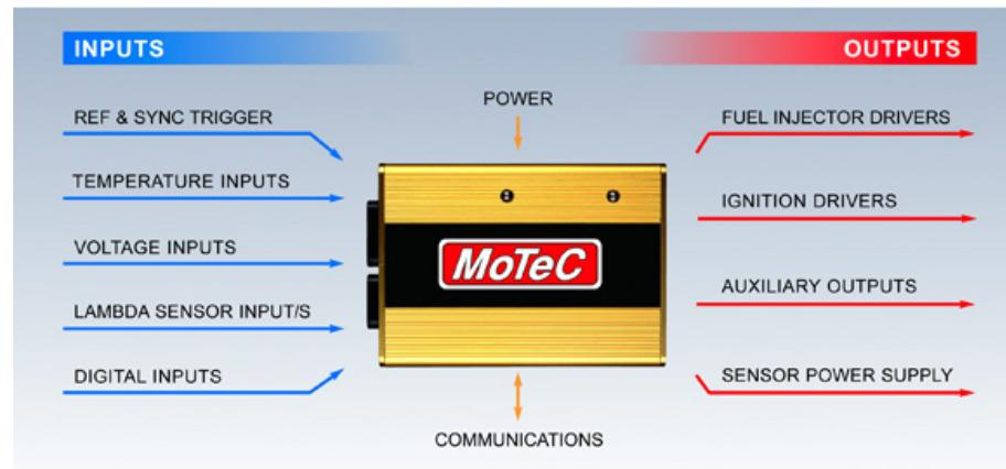
These are the main specifications of MoTeC's 'gold box' ECU range to compare the suitability of the different models for your application.
